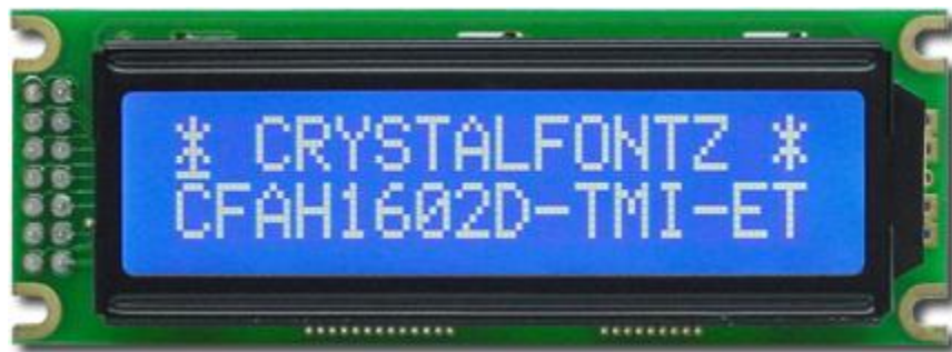
Figure 6.1: Crystalfontz 16x2 STN Negative Blue Transmissive White Edge LED Backlit LCD Module
